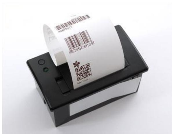
require any ink, but requires a special thermal paper for printing invoices. The device uses serial communication over UART for communicating with the microcontroller.
