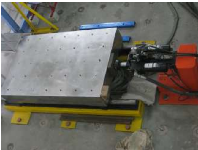
Uni-Axial Shake Table at the Structural Engineering Lab, IIT Kanpur
