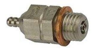
• Glow Plug plug filament needs to be heated up initially using a glow plug igniter(booster), once the engine is running the heat generated within the combustion chamber keeps the filament glowing continuously and is thus able to ignite the fuel/air mixture on each revolution.
